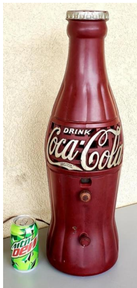
Figure #1: The 1933 Crosley Coca-Cola bottle radio. Tubes were located upside down on the bottom. Made of Durez which is a form of Bakelite hard plastic.
