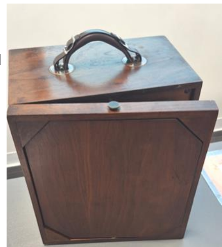
Radiola 26 with the lid partially open. The door contains a loop antenna that is rotatable and removable. The shape of the octagonal antenna is visible within the lid frame.
