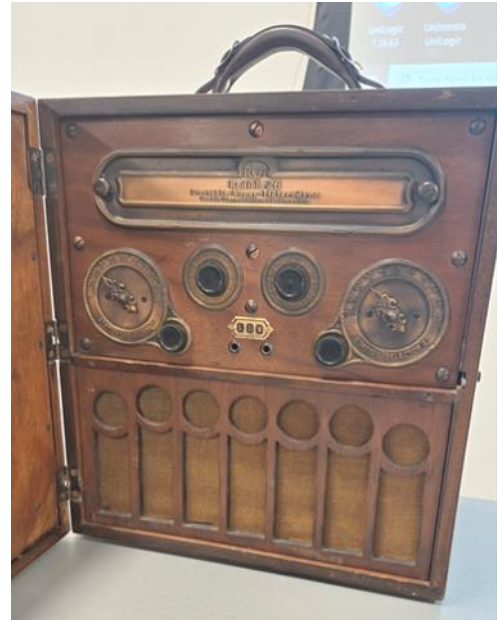
Radiola 26. The tubes are behind the removable brass colored metal oval cover at the top.
