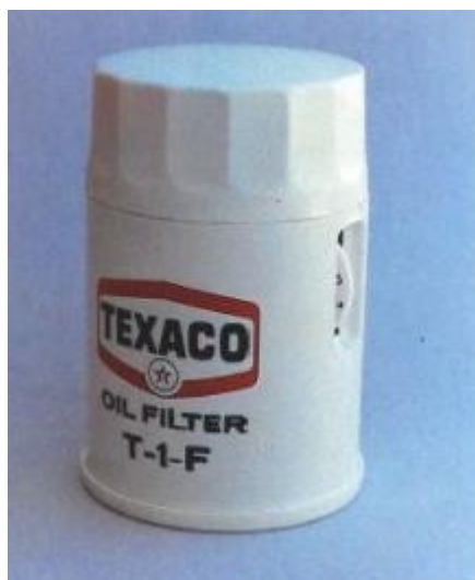
AM radio made to look like an automotive oil filter. This radio was sold at Texaco stations in the 60s and 70s. Speaker is on the bottom facing downward.
