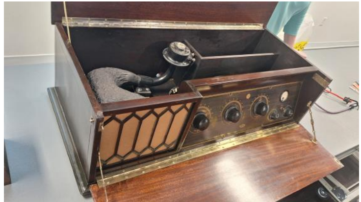
The radio with the front and top lids open. Notice the driver and speaker. The speaker is made of paper mache.
